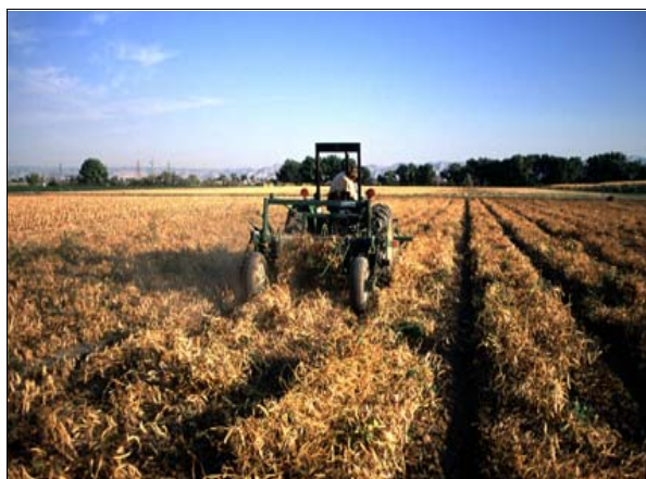
Fig. 1. Cutting dry beans at Fruita, Colorado in 2001 using a Pickett One-Step rod cutter windrower constructed for small plot research.
